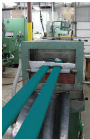
Raw Poly Lumber Exiting Extruder
