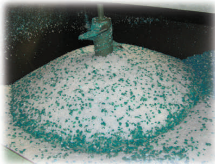
Raw Poly Beads Being Mixed In Auger
